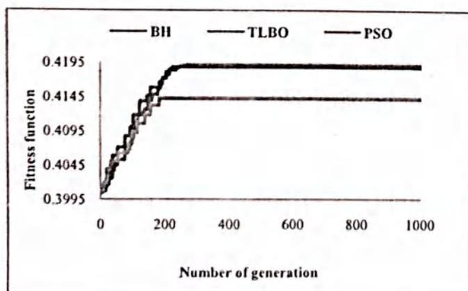
Fig. 1. Plot of convergence of fitness function with respect to number of generation using BH, TLBO & PSO algorithms for 14-bus system.
